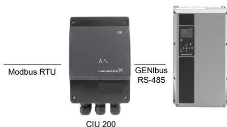
Principle sketch of CIU 200 Modbus RTU solution. The figure shows a CUE-drive for pumps
