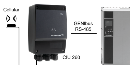
Principle sketch of CIU 260 Modbus cellular solution with external antenna. The figure shows a CUE-drive for pumps
