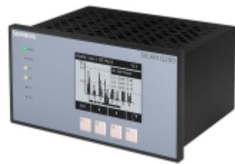
The device measures voltages up to 480 V in 1-phase systems and in 3-wire and 4-wire systems (with neutral phase). The input circuits for voltage measurement can be used in IT, TT and TN networks. To ensure galvanic separation for current measurements, the lines connected to the current measurement inputs are galvanically separated from the current transformers.
