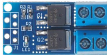
In these setups, the PWM supply voltage comes from the motor (shown by the blue-black wire in the diagram below), while the PWM signal is received on the brown wire. The Arduino operates at a 0-5 V signal level; in this case, the XY\_MOS signal converter can be used to match the two signal levels. Pay attention to this aspect:
