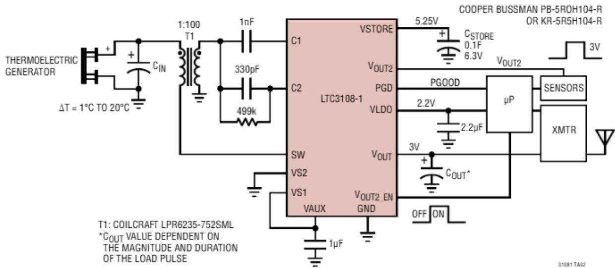
LTC3108-1, Voltage, Boost, Converter, power manager, step-up, DC/DC converter, thermoelectric generator, solar cell
