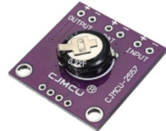
The Texas Instruments BQ25570 is intended for ultra-low power applications and lacks complex communication interfaces such as I<sup>2</sup>C, SPI, or UART. Instead, it relays status and control data through basic digital I/O pins and external resistor networks.
