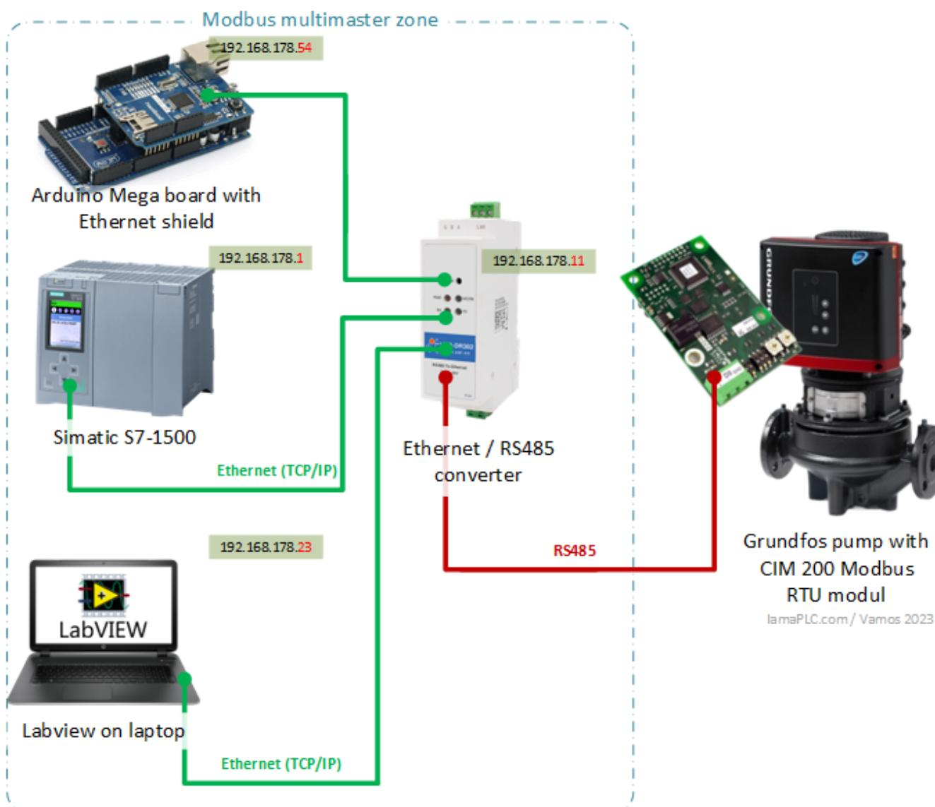
Through the CIM 200 module, the Grundfos pump can be controlled directly from the various controllers, and all its parameters can be read. These parameters can be displayed, for example, on HMI or SCADA. The Ethernet / RS485 converter converts TCP telegrams into RTU form and transmits them as such. Thanks to this unit, the connection can serve several master units (multimaster).
