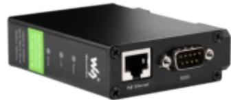
The rail-type case design, is small in size, easy to install, and cost-effective. It is very suitable for collecting the data of RS232/485/422 and sensors in the industrial field, including local network collection or uploading to the data that the cloud server autonomously collects and sends.
