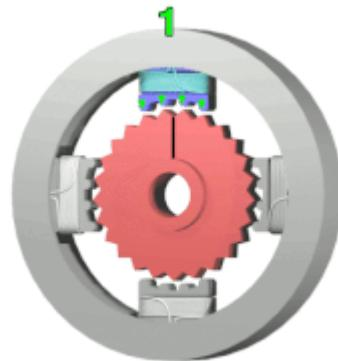
Switched reluctance motors are very large stepping motors with a reduced pole count, and generally are closed-loop commutated.
