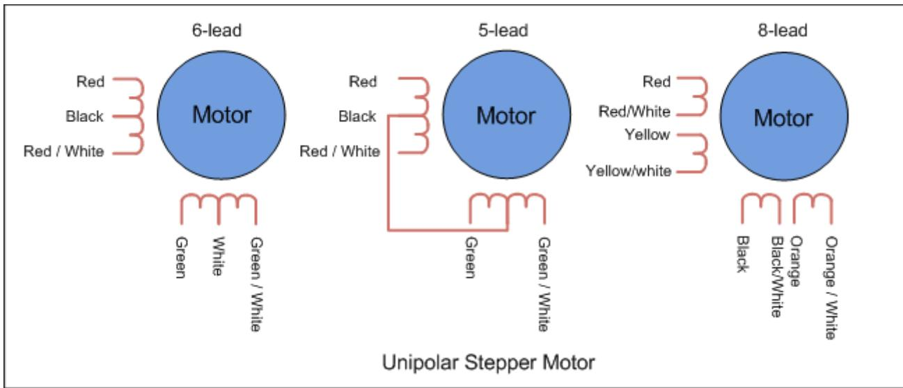
Typically, given a phase, the center tap of each winding is made common: three leads per phase and six leads for a typical two phase motor. Often, these two phase commons are internally joined, so the motor has only five leads.
