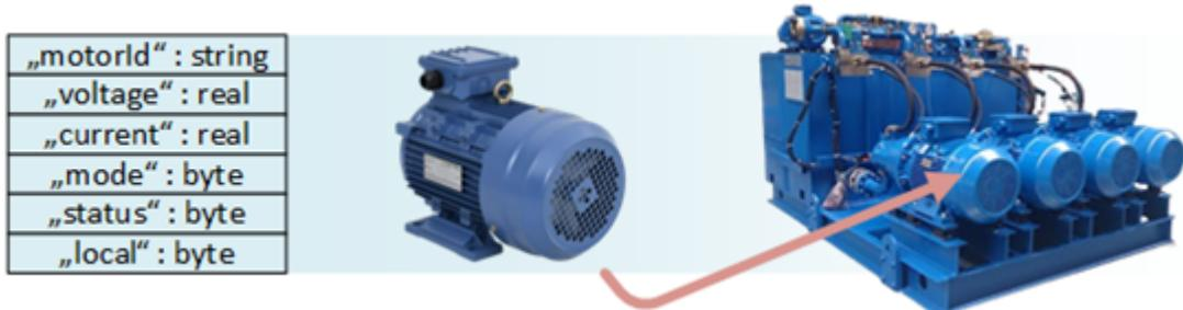
In this case, the motor has a text identifier, typically a KKS identifier in larger installations. Then there are voltage and current measurements, an operating mode, and a status indication. These data belong together and describe a motor. In the example above, this motor is, for example, the first motor of a hydraulic block. In the case of multiple motors, this structure remains—only the parameters change, as this makes it easy to handle the data uniformly:
