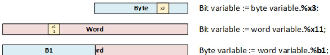
The following example is a SPLIT function that splits a WORD Input variable into bits:
