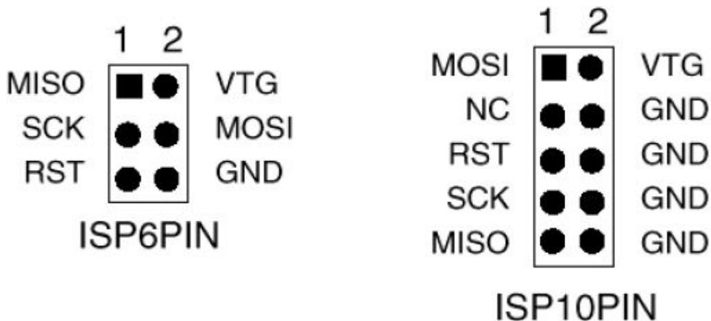
Additionally, these pins are connected in parallel with the corresponding pins of the IO ports (see below); therefore, they are grouped here for download convenience. It is also possible to use an Arduino board to upload programs to other Arduinos via the ISP (In-System Programming) method.
