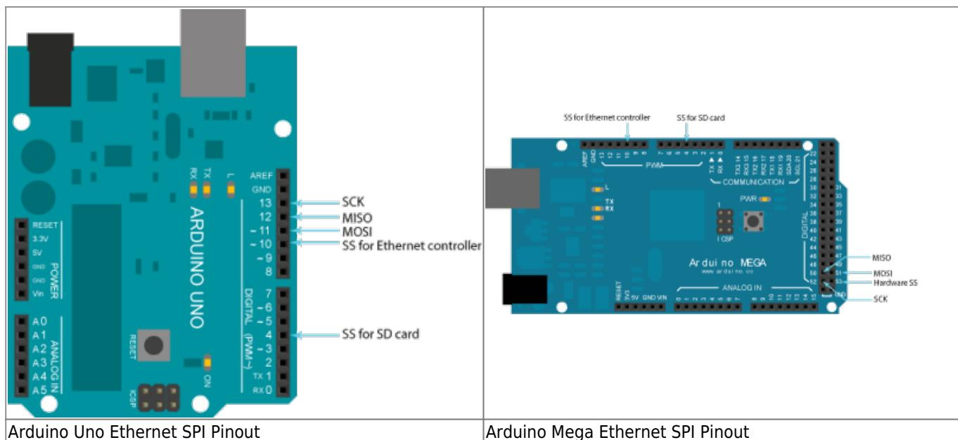
A micro-SD card reader is also integrated on most Ethernet boards. The use of this is optional, but it occupies an extra pin on the board.
